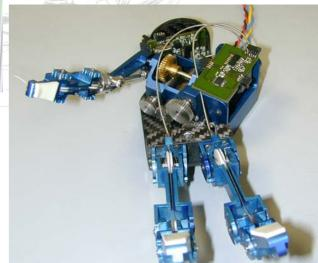
2 DC actuators (MINIMOTOR, CH) integrated in the palm
