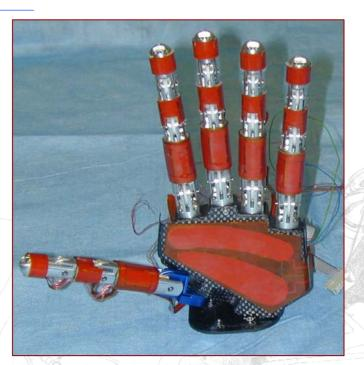
**15 Embedded Joint Angle Sensors (Hall effect)** (Operational range: 0 – 90 degrees, Resolution: ~0.1 degrees).
