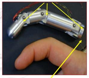
5 cable/tendon tension sensors (Operational range: 0 – 35 N, output characteristic: linear, resolution: ~20 mN)
