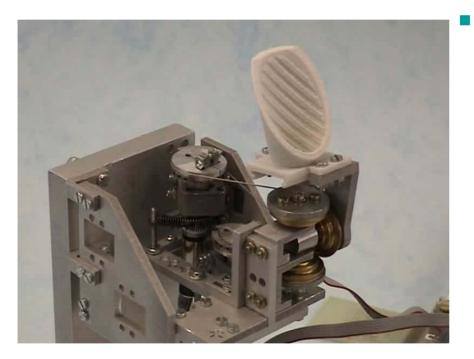
pre-tensioned cable driven differential mechanism, rotating the mounted pinna +/- 60 degrees with an accuracy of 0.1 degrees which exhibits practically no backlash
