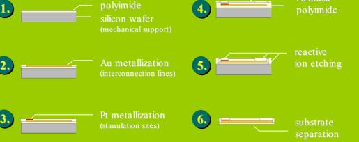
Technology process for the sieve electrodes implementation
