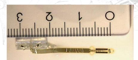
Sieve like electrode with tube and connector
