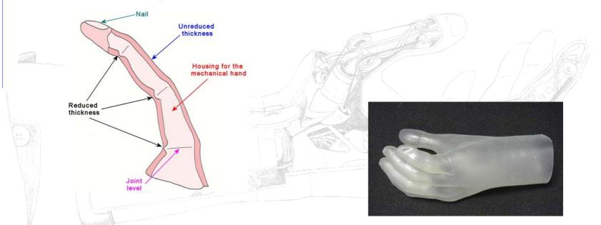
The first prototype of the cosmetic glove has been already fabricated and preliminary tested. The colour and other aesthetic details like nails, hairs, etc. have been not yet added.
