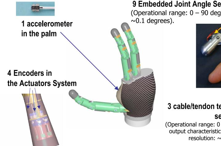
9 Embedded Joint Angle Sensors (Hall effect) (Operational range: 0 – 90 degrees, Resolution:
