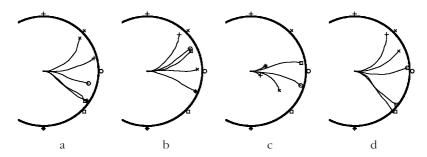
Figure 5. Unstable robot trajectories. Panels (a) and (b) were separated by 10 min, (b) and (c) by 5 min, and (c) and (d) by 1 min. The trajectories generated by the light marked with a star (\*), circle ( $\circ$ ), and square ( $\Box$ ) vary greatly from one trial to the next.
