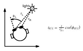
Figure 4. The response of the robot's sensors is a function of distance and angle from the light source.
