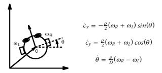
Figure 3. The dynamics of the robot are described by three nonlinear first order differential equations.
