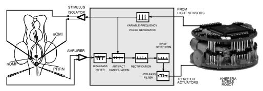
Figure 1. Block diagram of robot signal flow. The neuro-robotic interface (shaded center region) translates the light sensor data from the robot (right) into a stimulation pattern for the lamprey preparation (left). The neural response is converted into motor signals by the interface.
