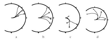
Figure 14. Sensor sensitivity was unilaterally doubled. Trajectories were recorded (a) before any changes in sensitivity were made, (b) immediately following this change, (c) after 5 min of steady stimulation, and (d) after a 5 min resting period.
