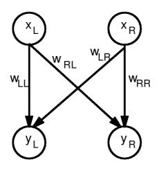
Figure 9. Simple two-layer neural network with two inputs, two outputs, and four weights.
