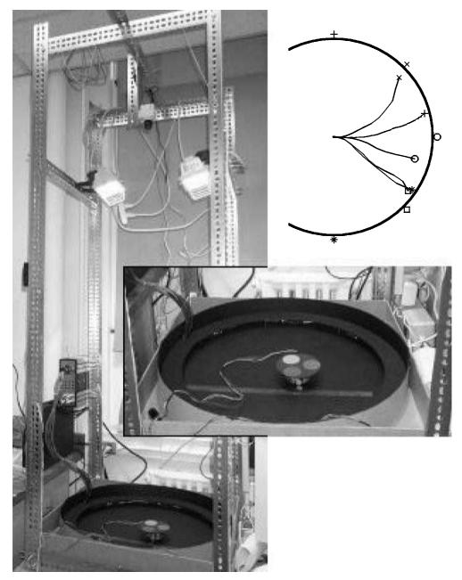
Figure 2. Robot setup. Using a pattern of colored disks (lower right), the overhead camera tracks the robot. Trajectories are plotted, each symbol representing a target light (upper right).
