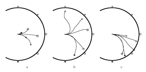
Figure 11. In these trials, the robot displays behavioral patterns that can be classified as: (a) negative, (b) positive, and (c) mixed phototaxis.
